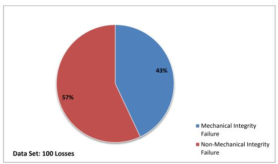
Mechanical integrity failure is a far more likely cause of major loss for refineries than for other occupancies as shown in Figure 4.
