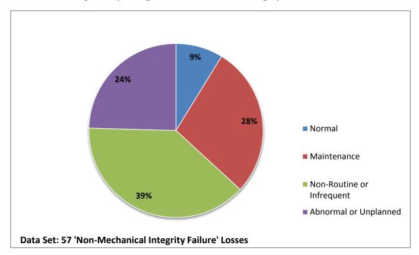
Figure 7 Operating Mode - 'Non-Mechanical Integrity Failure' Losses
